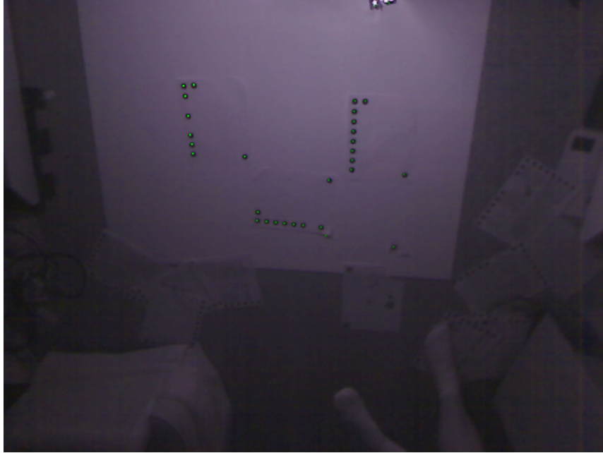
Figure 3.5: Raw output from camera with calculated fiducial dots overlaid in green.
