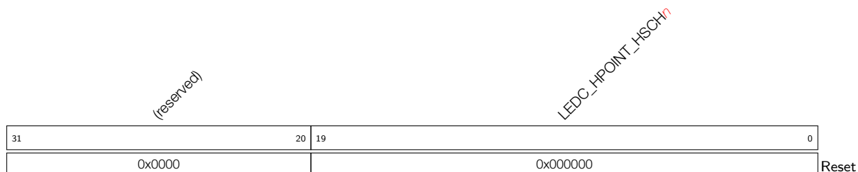
Register 10.2: LEDC_HSCH n _HPOINT_REG ( n : 0-7) (0x20+0x10* n )
